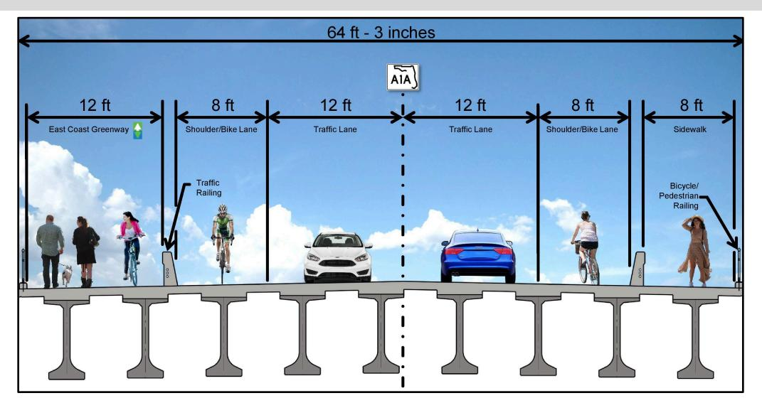
This picture shows a typical section of the new bridge.
