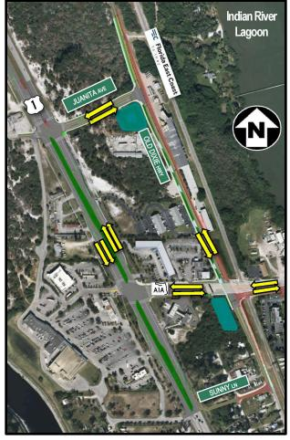
The yellow arrows show the flow of traffic during Phase 2 construction in Zones 1 & 2.
