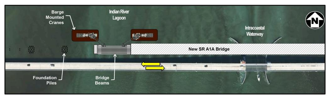
The yellow arrows show the open lanes of traffic in Zone 3 during Construction Phases 1-4.
