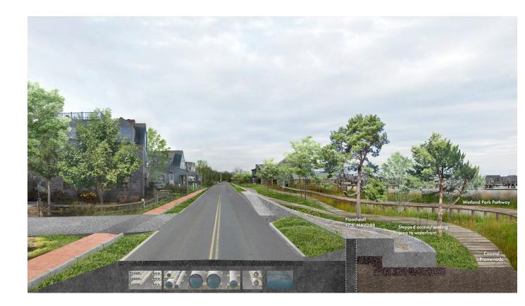
Above: Conceptual design of the Downtown Neighborhood Flood Barrier intended to reduce risk from future high tide flooding. This example shows a typical street condition, similar to Washington Street in Downtown. This is one way that a road elevation could serve as a barrier to flooding and be integrated within the character and experience of the Downtown streetscape.
