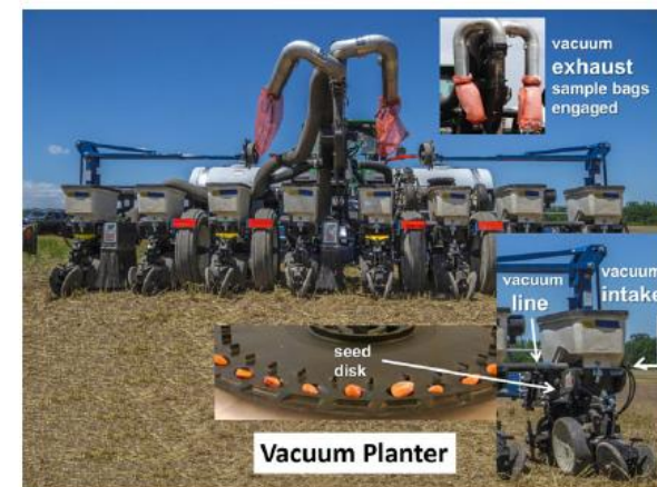
Figure 1. Kinze (Kearney Canada) vacuum planter showing exhaust location and dust collection device (top inset).
