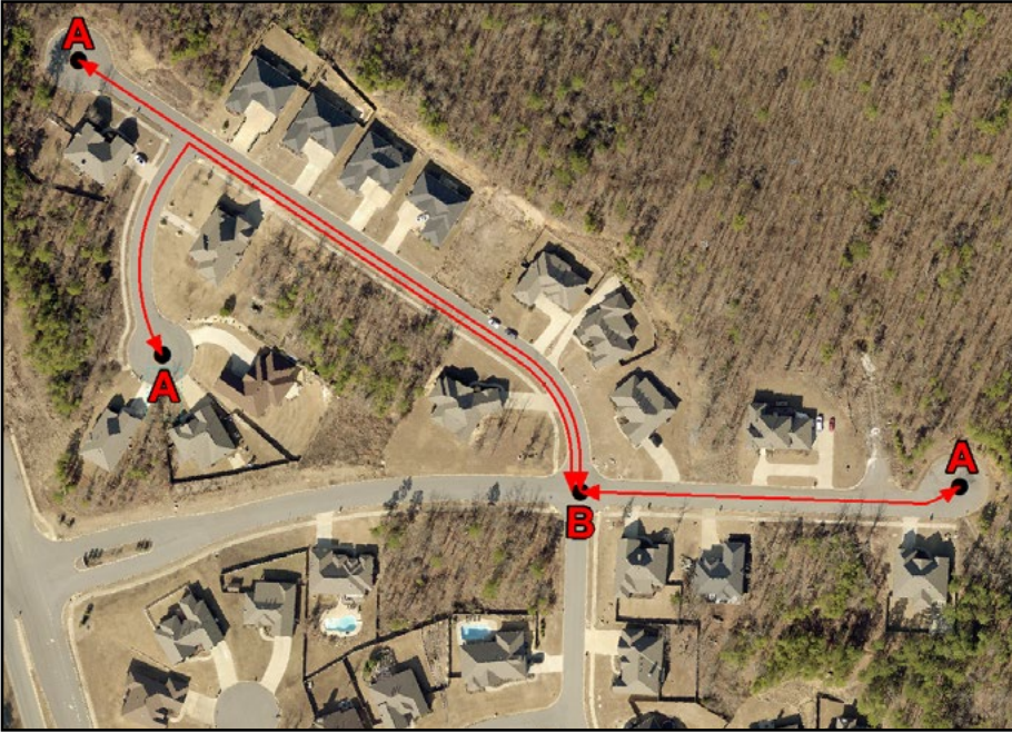
Figure 5.4.3.2.A. Measuring Cul-de-Sac Length
