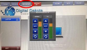
4: Turn on streaming to SD.net by touching the "SDPB Feed Off" button. Button will turn green when feed is active.
