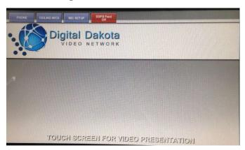
3: Ensure that the room mics are not muted, by tapping the "CEILING MICS" and the "MIC SETUP" buttons. Ceiling mics are not muted when green, and the wireless and lav mics are not muted when the Mute buttons are blue.
