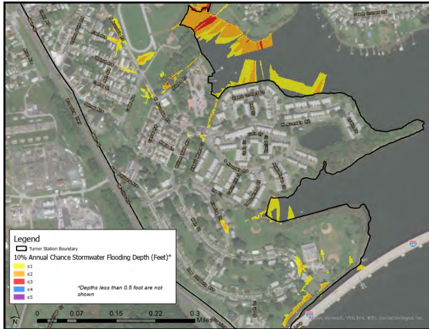
FIGURE 4.3: TURNER STATION SECONDARY AREAS AT RISK OF FLOODING – 10% ANNUAL CHANCE RAINFALL EVENT
