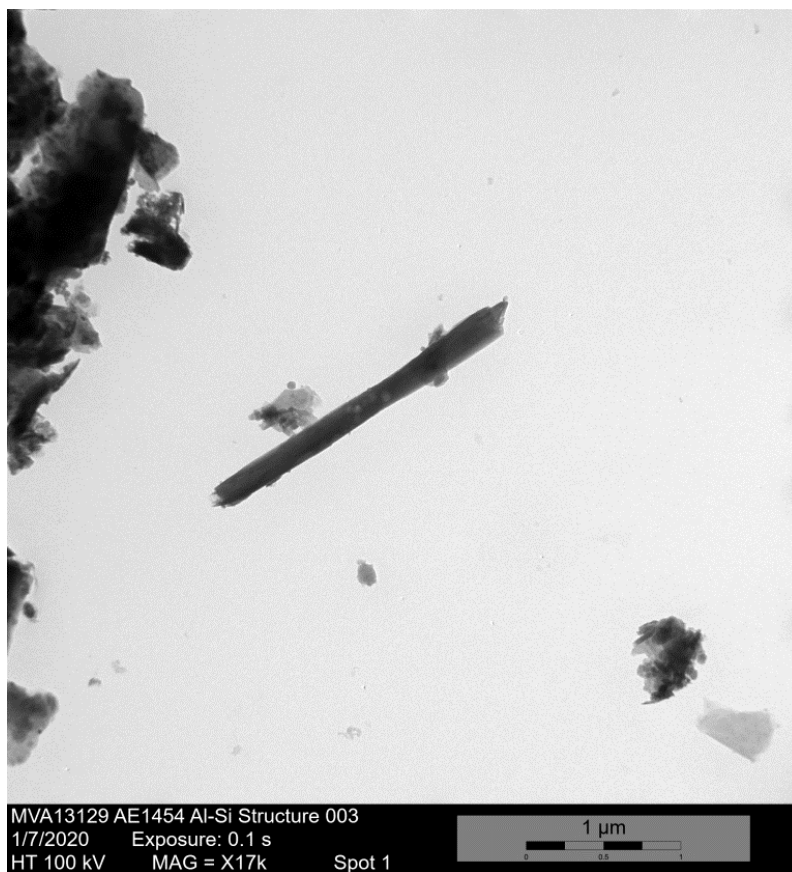
Figure 35. TEM image (above) and EDS spectrum (below) of representative fibrous silicate detected in the environment from air sample AE1454 (Test A – Pump #05).
