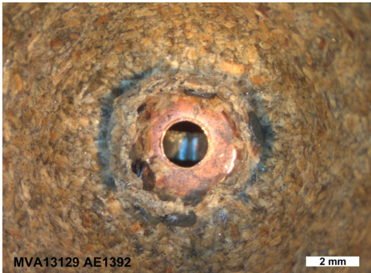
Figure 29. Stereomicroscope image of basewad in sample AE1392.
