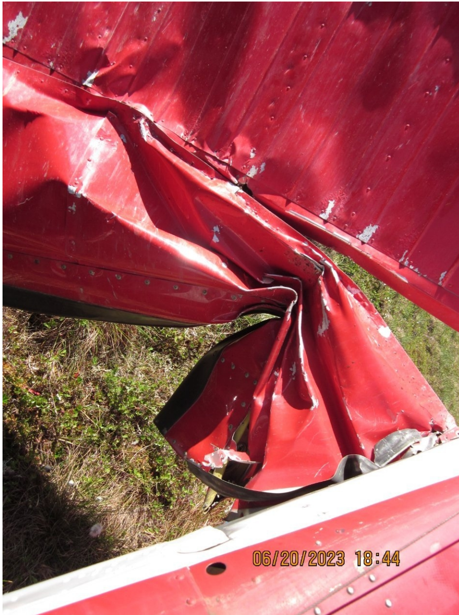
Figure 2. View of the aft crushing on the horizontal stabilizer.
