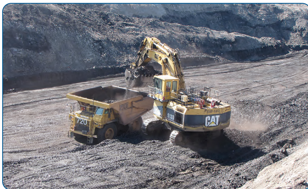
A coal shovel loading coal into a haul truck from a thin coal bed in the pit of a surface mine on Federal lands in the Yampa coal field in northwest Colorado. Photograph by David C. Scott, U.S. Geological Survey.
