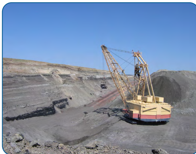
A dragline removing overburden rock from a thick coal bed in a surface mine on Federal lands in the Powder River Basin in northeast Wyoming. Photograph by the U.S. Geological Survey Coal Assessment Team.
