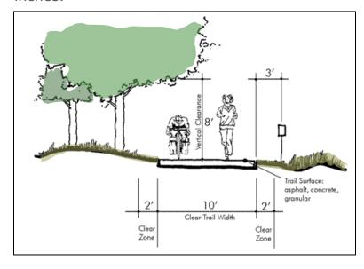
The cross section of the trail shall be sloped at a maximum of 2%, the maximum grade for all trail sections shall not exceed 5%.
