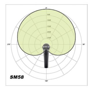
You'll notice that the microphone's sensitivity is the lowest at the base of the microphone, where its cable plugs in. This means that sounds coming from "behind" the microphone are picked up the least, and this is where rejection is the highest.
