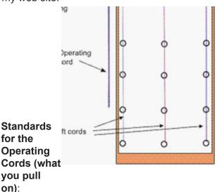
There cannot be a hazardous loop when the shade is in the fully lowered position. If a cord connector is used (this can simply be a knot) the lift cords must be braided or completely separate. If no cord connector is used, the cords must be completely separate. If a loop cord is used it must be attached to the wall using an approved break-away tension device.
